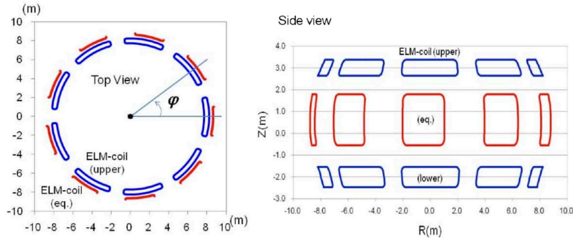
Figure 1 Geometry of ELM mitigation coils in ITER
